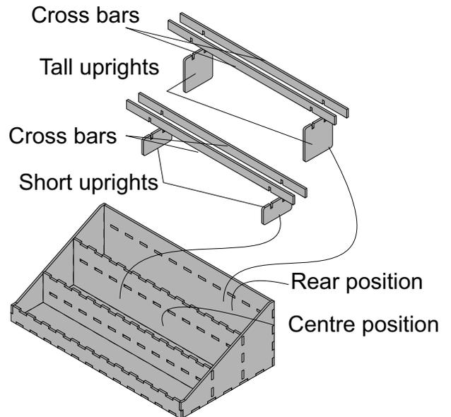
**1:** Place short and tall inner panels into the base first. Glue side panels into place followed by the back and front panels.
