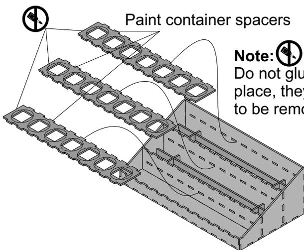
**3:** Place paint jar spacers into the slots on the back panels. Spacers are designed with a breakaway tab to allow for larger paint containers.
