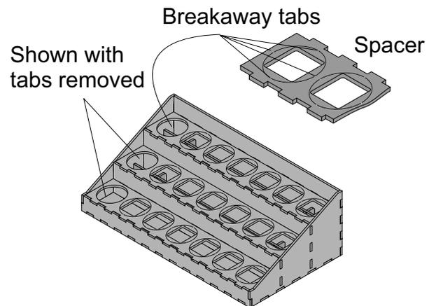
**4:** Once assembly is completed you may want to seal your work station using urethane or an epoxy resin.
